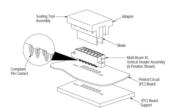
Seating Tool Assemblies 1725769-[] For Multi-Beam XL Vertical Header
